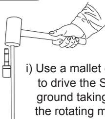
i) Use a mallet or lump hammer to drive the Spike fully into the ground taking care not to hit the rotating male Pole connector.
